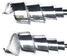
Fig. Good chip control (A7075)
